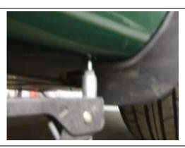
6. Fit the 10 off M5 rubber ankernuts into the fibre glass sill as shown each side.
