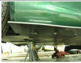
Unbolt the three forward rear mid floor section side mounting bolts each side. Then offer the side sill up in place and re-fit with three c/sunk bolts and alloy c/sunk washers (supplied).
