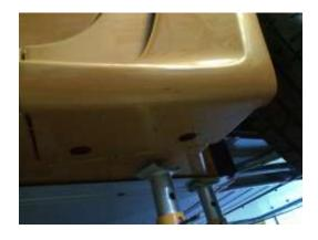
5. Fit the 2 off M6 c/sunk 40mm bolts and bevel washers in place of the lotus front fender lower bolts. Do this on both sides of the car. Once happy drill through into the GRP sill carefully! (oil pipes present!) through the additional holes in the panel, use a 4mm then a 9mm drill bit..
