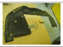
3. Old OEM spoiler Removed with steel insert
