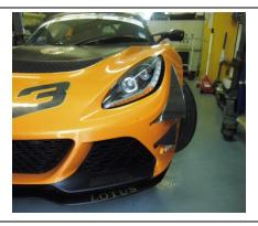
Bolt canards in position with 4 off M5 bolts and washers supplied. Refit inner arches and wheels and lower vehicle to ground carefully.
