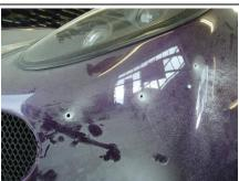
4. Offer front canards in position and drill four 5.5mm fixing holes each side.
