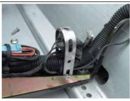
2. Make slotted bracket as shown with M5 Rivsert fitted. Steel slotted and drilled Strip Bracket material can be sourced on-line or motorists supply stores.
