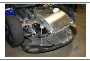
5. Alloy ducting fabrication shown in position around ProRad from sector111.com in USA. Reverie do not make or supply the GT3 style inlet and exit shrouds which were originally made by Lotus cars for racing.
