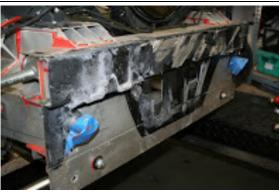
2. Remove glass fibre crash structure using cheese wires or vibrating knifes to try and cut through adhesive. Or simply cut through fibre glass and then slowly and carefully grind back crash structure till bond and eventually alloy just exposed.
