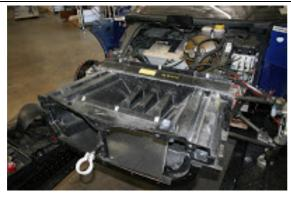
1. Loosen wheel bolts. Jack up car carefully following lotus owner's manual instructions for correct procedure. Support on axle stands. Remove wheels and plastic inner arch liners and front clam shell. Remove radiator and all pipe work.
