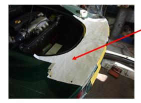
TAPE IN PLACE ON THE REAR CLAM THE PROVIDED DRILLING TEMPLATE
