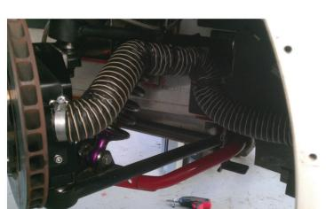
If you use the Elise Parts uprights we can create race spec hub mounted brake cooling products as per picture
