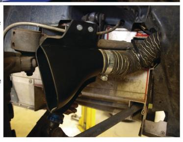
Bell housing offsets and rotor sizes vary massively depending on application and specification, which is why we have ended up with this generic (best case scenario for all elises) disc bell air canal and mounting design.
