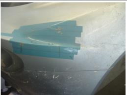
Cover the area shown in photo in pvc insulation tape
