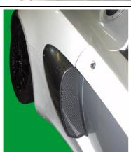
8. Optional outer carbon side ducts shown. N.B with holes for Exige S2, without holes for Elise S2. See <a href="https://www.reverie.ltd.uk">www.reverie.ltd.uk</a> for details. Refit the inner wheel arch liners and refit the road wheels. Lower car to the ground and torque wheel nuts.
