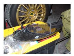
3. New reverie outer duct shown ready to be fitted. Note rear tag to go to existing bolt, lower strap to go to std posi drive fixing hole, front tag which drops over rubber edge trim and top tag which requires one 3mm hole to be drilled in body work and a posi screw fixing.
