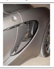
1. Chock front wheels, Jack up rear of car and remove road wheels. Remove the rear inner wheel arch liners and standard plastic side duct, see instructions for removal in outer ducts section 1.
