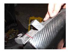
5. O.e plastic grille shown fitted behind our new outer scoop. If an oil cooler is fitted or for other reasons you do not wish to keep the o.e plastic grille then simply cut the forward upper section off along the red line shown. This small piece can then be bonded in situ with a small amount of PU adhesive around the tag. Again always do this once the outer scoops forward upper fixing is secured (see 6/7).
