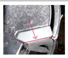
4. If fitting the outer ducts with no inner duct then the grille finishes in the door shut at the red line shown in the image, leaving a hole above. This is best remedied by either fitting our inner scoop, or refitting the whole of the o.e plastic grille behind the outer scoop. Either way always affix the upper forward outer scoop tag first (see 6/7), then slide the replacement inner scoop or o.e part in from behind.
