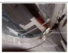
6. Push the new reverie duct through the rubber from the outside, having lipped the front lower tag over the rubber.
