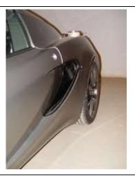
3. External View of Air inlet feed duct (optional) Fitted alone.
