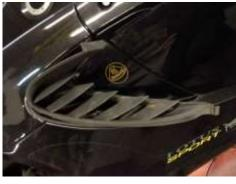
1. Clock the front wheels, jack the rear of the car up, and remove the rear road wheels. Remove the rear inner wheel arch liners and standard plastic grilles. There is a fixing point at the rear inside (10mm spanner req), and also a posi self-tapping screw again also inside.
