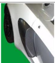
8. Optional outer carbon side ducts shown. N.B with holes for Exige S2, without holes for Elise S2. See <a href="www.reverie.ltd.uk">www.reverie.ltd.uk</a> for details. Refit the inner wheel arch liners and refit the road wheels. Lower car to the ground and torque wheel nuts.
