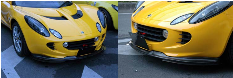
S2 spoiler fitted in position
