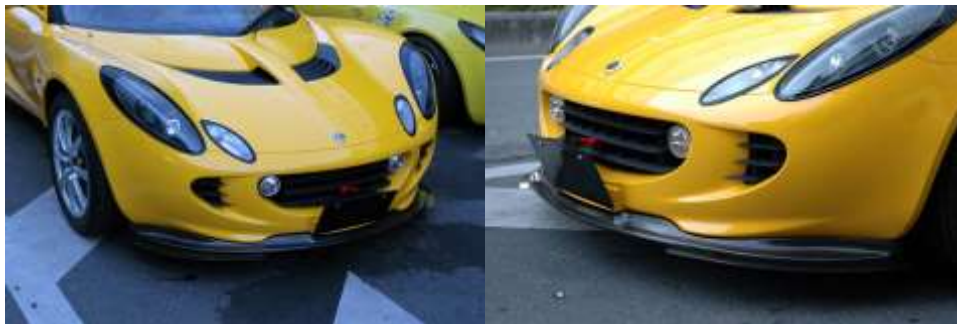
S2 spoiler fitted in position
