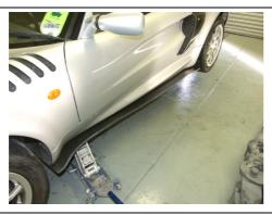
7. Carefully lower the car to the ground. **Then importantly** for best appearance push the rubber edging on so that the seen side fits snugly without creases, this will leave the non seen underside slightly creased. This rubber edging has been bonded using a super glue adhesive just along the centre length.
