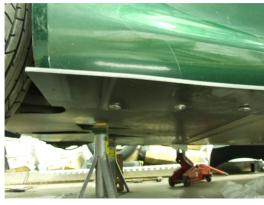
2. Unbolt the three forward rear floor section side mounting bolts each side. Then offer the side sill up in place and re-fit with three c/sunk bolts and alloy c/sunk washers (supplied).
