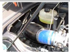
13. Push Samco 45' angled hose into position and clamp both ends. Rotate 45' elbow as required to best position Daytona canister.
