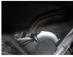
S2 - Trumpet cable tied in position to gain maximum air from side vent. S1 100mm duct clipped over 100mm side vent exit snorkel
