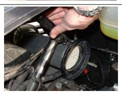
Push flat stepped diffuser duct into end of side vent 100mm duct and tighten clamp.
