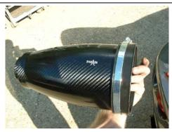
12. Push filters with extension moulding into Daytona canister and tighten clamp. Push Flat stepped diffuser and Daytona canister filter end together and tighten 2<sup>nd</sup> clamp on filter end.
