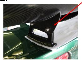
Bolt the Alloy Wing mounts to the wing at a mid angle of attack position. The carbon wing supports outer sides should be approx 900mm apart. Then sit the wing and supports carefully on the boot, Centralise the wing on the boot using the lines on the template as reference to help. Check the boot can open if using the curved wing profile. Check the holes marked are in the right position if not then re-mark them in a new position you are
