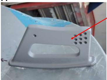
Now drill through the 4 clamshell mounting holes into the carbon curved 90' support of the internal carbon/foam boot strengtheners. Inject some silicone into the top 4 clamshell holes to stop water ingress. Stick some 3mm self adhesive neoprene to the underside of the alloy supports and trim around with a sharp knife. Next bolt the alloy supports in place and refit the wing.
