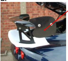
Bolt the Alloy Wing mounts to the wing at a mid angle of attack position. Then sit the wing and supports carefully on the boot, Centralise the wing on the boot using the lines on the template as reference to help. Check the boot can open if using the curved wing profile. Check the holes marked are in the right position if not then re-mark them in a new position you are happy with.
