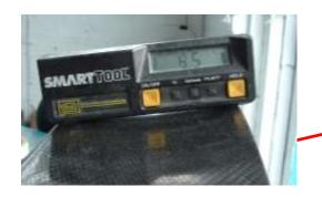
WITH THE VEHICLE ON A FLAT SURFACE AND THE RIDE HEIGHT EQUAL ALL-ROUND, SET THE WING TO THE ANGLE OF ATTACK YOU REQUIRE. TUNE THIS AT A RACE CIRCUIT OR WIND TUNNEL TO GIVE A NEUTRAL AERO BALANCE. NOTE ADD APPROX 2 DEGREES TO THE READING AS IT SHOULD BE TAKEN TO THE CENTRE OF FRONT WING RADIUS NOT TOP.
