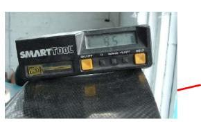
WITH THE VEHICLE ON A FLAT SURFACE AND THE RIDE HEIGHT EQUAL ALL-ROUND, SET THE WING TO THE ANGLE OF ATTACK YOU REQUIRE. TUNE THIS AT A RACE CIRCUIT OR WIND TUNNEL TO GIVE A NEUTRAL AERO BALANCE. NOTE ADD APPROX 2 DEGREES TO THE READING AS IT SHOULD BE TAKEN TO THE CENTRE OF FRONT WING RADIUS NOT TOP.
