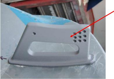
Now drill through the 4 clamshell mounting holes into the carbon curved 90' support of the internal carbon/foam boot strengtheners. Inject some silicone into the top 4 clamshell holes to stop water ingress. Stick some 3mm self adhesive neoprene to the underside of the alloy supports and trim around with a sharp knife. Next bolt the alloy supports in place and refit the wing.
