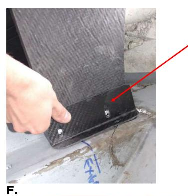
Position the 90' carbon lower bracket along the bottom inside edge on elise S2 (outside i.e behind on Exige S2) and Then mark the hole positions required in the mount to match those in the floor of the boot (Elise and Exige are different, See section G). Next drill 8mm holes in the base. Then bolt the bracket in place to the supports and boot floor/chassis. (ELISE CLAM SHOW!)
