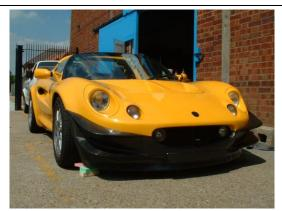
1. Remove front number plate plinth Trial fit spoiler with 2 people, one each side as the wheel arch return lip has to be sprung over.
