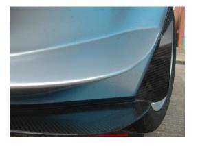
7. Optional front tyre deflectors R01SB0152 can also be riveted onto the arch lip return each side to provide further front down force with little drag penalty.
