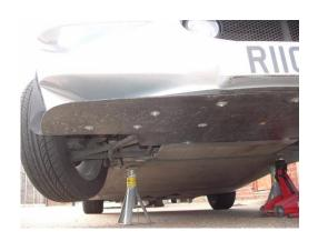
6. With the car carefully jacked up fit the splitter plate with shiniest surface upper. Use large washers and longer retaining m5 bolts as required to temporary fit.
