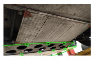
4. View underneath car where optional front splitter R01SB0102 can be fitted, original M5 fixings circled.
