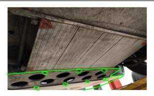
1. View underneath car where front splitter R01SB0102 can be fitted, original M5 fixings circled.
