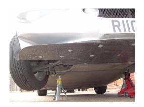
2. With the car carefully jacked up fit the splitter plate with shiniest surface upper. Use large washers and longer retaining m5 bolts as required to fit, loosely bolt in place with the three rear fixings and one further forwards centre fixing
