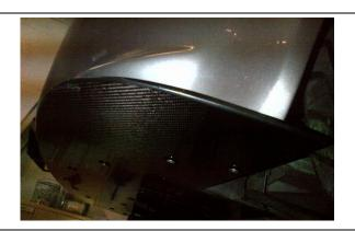
3. Splitter shown up in position and fully bolted up with top hats etc. All the original holes and fixings should be M5, the 5 new additional fixings along the front are M6
