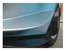
4. Optional S1 front tyre deflectors R01SB0152 can also be riveted onto the arch lip return each side to provide further front down force with little drag penalty.
