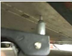
6. Fit the 3 off M6 alloy rivserts into the chassis as shown.
