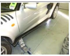
8. Carefully lower the car to the ground. **Then importantly** for best appearance push the rubber edging on so that the seen side fits snugly without creases, this will leave the non seen underside slightly creased. This rubber edging has been bonded using a super glue adhesive just along the centre length.
