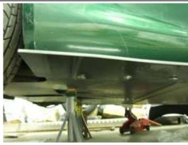
Unbolt the three forward rear floor section side mounting bolts each side. Then offer the side sill up in place and re-fit with three c/sunk bolts and alloy c/sunk washers (supplied).
