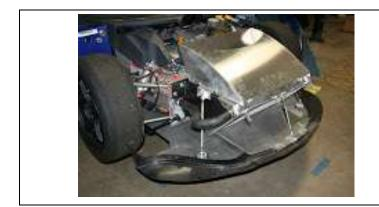
5. Alloy ducting fabrication shown in position around ProRad from sector111.com in USA. Reverie do not make or supply the GT3 style inlet and exit shrouds which were originally made by Lotus cars for racing.
