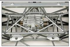
2. Offer up the diffuser and mark for any suspension cut outs or chassis bracket cut outs as required. Then wearing eye protection, ear defenders and a fine dust mask, cut the required cut outs with 3" thin carbide cut off wheel in a right angled grinder. You can use a hole saw to neatly end any wishbone arm cut outs required. Carefully dress and sand the sharp edges of any cuts made.
