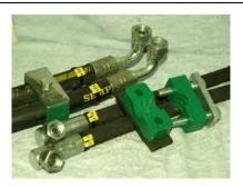
4. Obtain plastic hydraulic type hose clamps to suit chassis diameter tubing where required to give a firm fixing. Note these are also often used on race cars as anti roll bar clamps or sway bar clamps. These can be purchased from http://www.merlinmotorsport.co.uk/SUSPENSI
