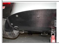
5. Check full bump and droop suspension clearances on tyres and wishbones with a spring professionally removed from the shock and the shock unit re fitted so you can see full bump and droop. Then ensure all bolts tight and the diffuser is fixed so rigid as any movement will effect aerodynamic performance. Carefull lower to ground and check wheel torques and tyre clearance again before carefully test driving to ensure all ok.
