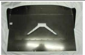
6. View of underside of diffuser for SV De Dion chassis, not fitted.
