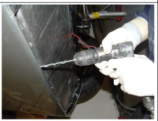
3. Drill the chassis and diffuser for required fixings, the chassis can be opened up and have m5 threaded rivserts fitted or in some areas if the tube is thick enough drilled and taped or rivets and washers under head may be used to secure in position, other options include using hydraulic clamps see 4.
