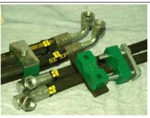
4. Obtain plastic hydraulic type hose clamps to suit chassis diameter tubing where required to give a firm fixing and save drilling the chassis tubes. Note these are also often used on race cars as anti roll bar clamps or sway bar clamps. These can be purchased from <a href="http://www.merlinmotorsport.co.uk/SUSPENSION-Associated-Suspension-Parts-Roll-Bar/c31">http://www.merlinmotorsport.co.uk/SUSPENSION-Associated-Suspension-Parts-Roll-Bar/c31</a> 32 33/index.html
