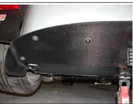
8. Check full bump and droop suspension clearances on tyres and wishbones with a spring professionally removed from the shock and the shock unit re fitted so you can see full bump and droop. Then ensure all bolts tight and the diffuser is fixed so rigid as any movement will effect aerodynamic performance. Carefully lower to ground and check wheel torques and tyre clearance again before carefully test driving to ensure all ok.
