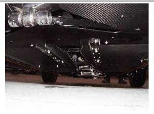
Diffuser shown fitted in place with De-dion axle arm in full droop coming through diffuser cut out.
