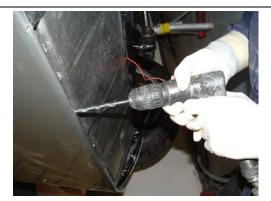
3. Drill the chassis and diffuser for required fixings, the chassis can be opened up and have m5 threaded rivserts fitted or in some areas if the tube is thick enough drilled and taped or rivets and washers under head may be used to secure in position, other options include using hydraulic clamps see 4.
