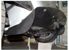
7. Diffuser shown fitted in place with De-dion axle arm in full droop coming through diffuser cut out.
