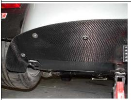
9. Check full bump and droop suspension clearances on tyres and wishbones with a spring professionally removed from the shock and the shock unit re fitted so you can see full bump and droop. Then ensure all bolts tight and the diffuser is fixed so rigid as any movement will effect aerodynamic performance. Carefully lower to ground and check wheel torques and tyre clearance again before carefully test driving to ensure all ok.
