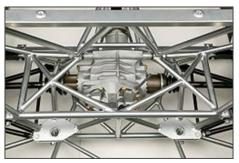
2. Offer up the diffuser and mark for any suspension cut outs or chassis bracket cut outs as required. Then wearing eye protection, ear defenders and a fine dust mask, cut the required cut outs with 3" thin carbide cut off wheel in a right angled grinder. You can use a hole saw to neatly end any wishbone arm cut outs required. Carefully dress and sand the sharp edges of any cuts made. (Sorry independent rear car shown)
