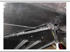
6. Diffuser shown fitted in place with De-dion axle arm in full droop coming through diffuser cut out.
