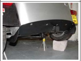
8. Diffuser shown fitted in place with De-dion axle arm in full droop coming through diffuser cut out.
