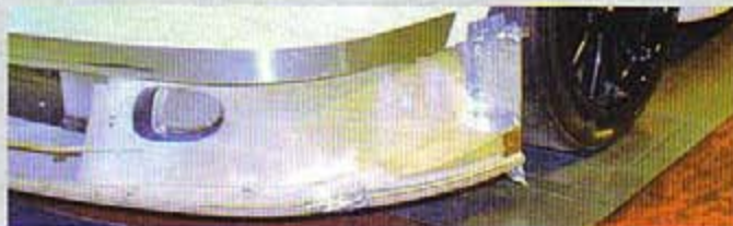
The airdam/splitter configuration seen on the BTCC Honda Touring Car that inspired this month's wind tunnel trials
