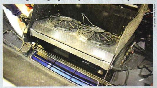
The initial radiator and ducting on the Britcar Noble. Improvements made to this installation included raising the angle of the radiator nearer to vertical so the pressure drop across it created less lift force and less obstructive supports for the fans that blanked off less radiator area. Both sought to reduce drag and increase front downforce
