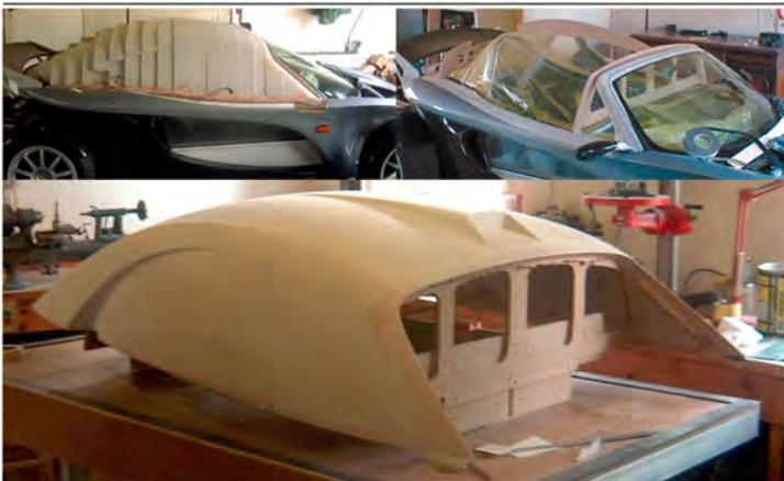
Sections were plotted, & then cut from 100mm styling foam block. This was assembled, hand shaped & trial fitted through the different stages. The pattern was then painted & weired up ready for manufacture of split tooling.
