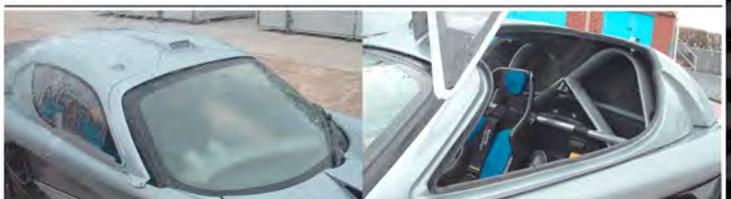
Careful attention was paid to the design of door guttering to ensure sealing of door rubber & good drainage. The complete perimeter was sealed to give tested effective weather protection. The hardtop was also extensively tested at high speeds.
