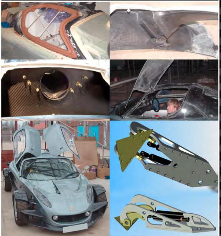
Gutter returns were modelled in clay to allow modification of the tool. A centre spine was produced combining centre roll hoop fixing & ram-air induction. A dihedral door system was selected & an initial prototype hinge was produced. This was CAD modelled to be produced in machined alloy.
