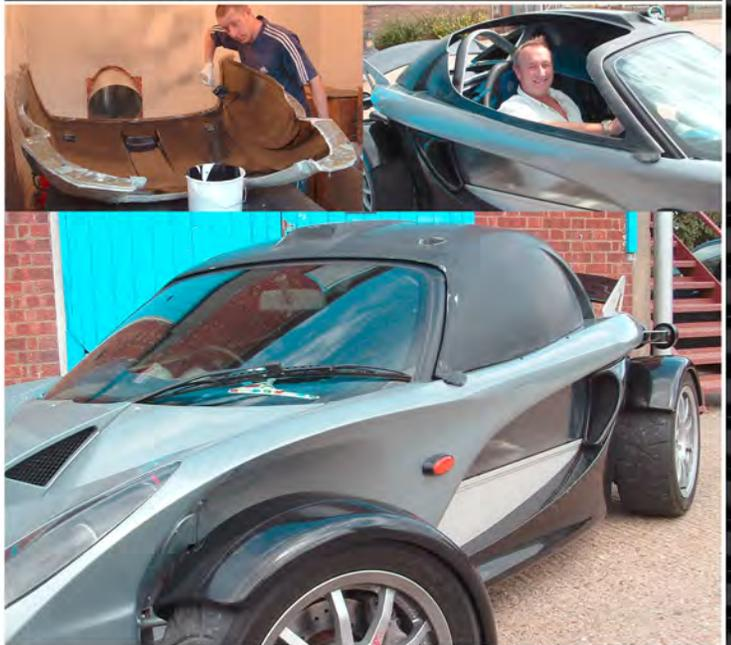
A GRP prototype tool was made from the hardtop pattern with no door gutters. A part was made from the tool & successfully trialed & fitted to a 340r. The door aperture was then cut & access tested.
