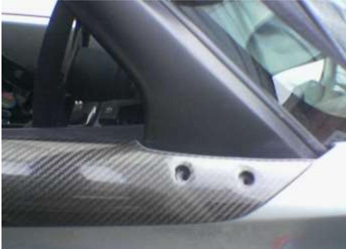
The rear can be bonded down with Sikaflex or similar or a super strong Velcro or double sided tape adhesive. Then rebolt the Mirrors and spacers on with longer bolts at the front.
