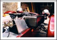
9. Bolt the backplate to the carbs/throttle bodies with the inlet trumpets in place or push the trumpets into silicon hoses and clamp as appropriate. Refit the airbox and ensure there are no foul conditions. Where the airbox protrudes through the bodywork small amounts of trimming might be required if the airbox is larger than the previous foam filter.
