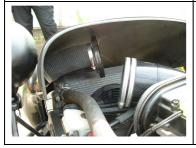
18. As the nose fairing hinges down into place it should be easy to locate the inlet cap into the rubber extension moulding on the cone air filter. Once in position and pushed fully home, tighten the hose clip to hold the inlet cap in position. Connect the engine management MAP air pressure sensor to the airbox with a length of 4mm vacuum hose through a grommet in the backplate.
