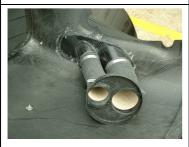
15. The 58 & 75mm lengths of micropore ducting are used to connect the snorkels to the 'Daytona' inlet cap. These can now be connected and held in position with the hose clips provided.
