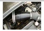
11. It is now possible to locate the 'Daytona' filter canister. ReVerie suggests cable tying this item to the 'X' brace to the rear of the anti-roll bar (as shown). To minimise any problems of wear and rattle it is recommended that a small amount of self adhesive foam is applied to the chassis frame in this area. The canister connects to the Airbox via a short length of micropore ducting (as shown).
