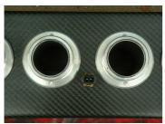
7. Some throttle bodies, including Weber Alphas, require the trumpet bases to be pressed off the trumpets. The bases are often bonded in place and heat might need to be applied to weaken the adhesive. Once apart the trumpets can be pushed through the carbon backplate before being rebonded (with DP490) and pressed back together. In the case of the Weber Alpha system, the trumpet bases are threaded allowing direct fixing to the backplate via bolts.
