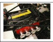
1. Remove existing air filter from the engine and leave trumpets attached to throttle bodies/carbs.
