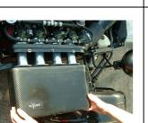
4. Offer up the airbox without its backplate to check for clearance. It is possible that the airbox may require some trimming to ensure it doesn't foul the front mudguard on full lock. Use of a template might make visualisation of this easier. Once happy that sufficient space is available bolt the airbox to the backplate ready for the next stage of fitting. Note that there should always be at least a 25mm gap between the airbox and trumpet mouths.
