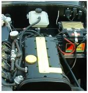
To allow for the installation of the induction system it is necessary to move the coolant bottle from its original position. ReVerie recommends mounting it on the engine bay bulkhead and lengthening and altering the coolant hoses, as shown.
