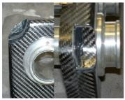
10. The Weber Alpha throttle bodies cause the standard ReVerie XE backplate to interfere with the throttle cable. This might also be the case with some other systems. If the kit is ordered for the Weber Alpha system the backplate will be supplied with a minor modification to allow clearance (as shown). This is simply achieved cutting away the section causing a problem and bonding thin, flexible flat sheet carbon in place with DP490.
