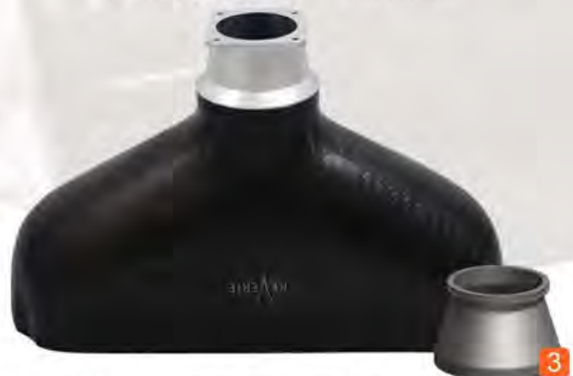
Fontana 112X Turbo or N/A plenum, 275mm total depth from back plate mounting surface. Volume: 8.0L
