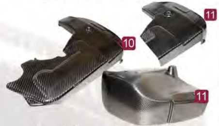
Cam belt cover for Ford YB cosworth available as full or half cover, fully EMI shielded uses OEM fixings
