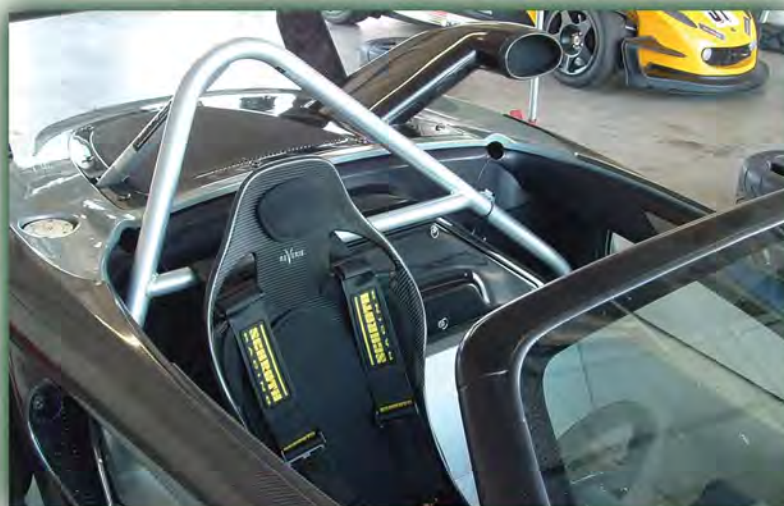
Mulsanne B light weight single skin, carbon fibre seat Mass: 3.0kg (approx) R01SI0017
