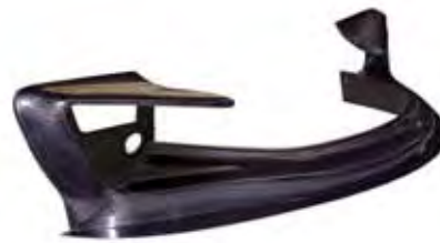
340R carbon fibre / GRP deep spoiler, includes splitter plates and gurney end plates with brake ducts Carbon fibre R01SB0051 GRP R01SB0052 (See images left and page header)
