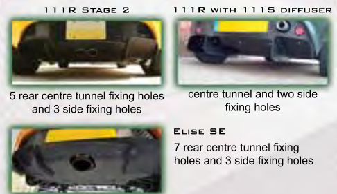
7 Three element for all models, 3.20kg, use with wider midfloor sections, available undrilled or with 3/5 centre tunnel fixing holes Undrilled R01SB0253 3 holes R01SB0251 5 Holes R01SB0252
