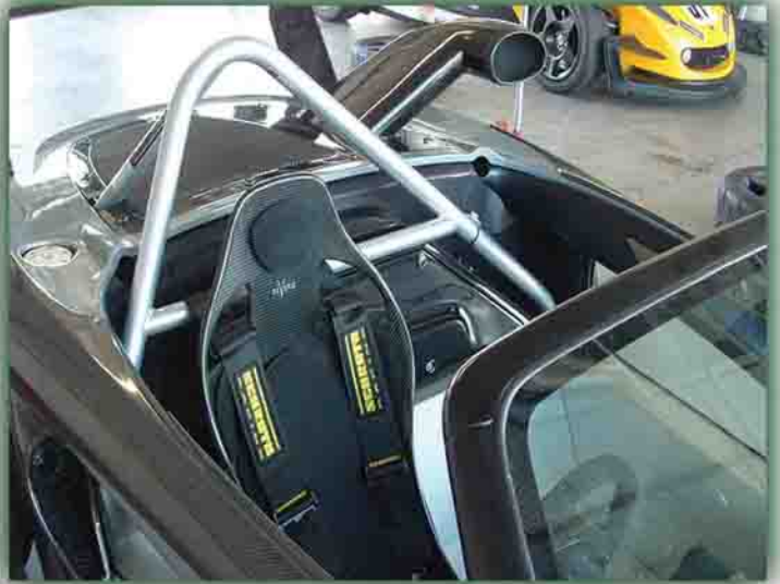
3 Mulsanne B light weight single skin, carbon fibre seat Mass: 3.0kg (approx) R01SI0017
