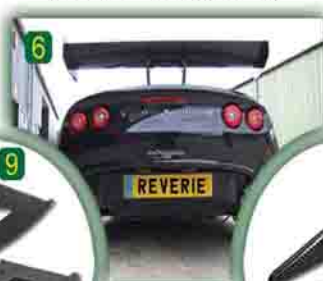
Fixed tailgate mounted straight wing
