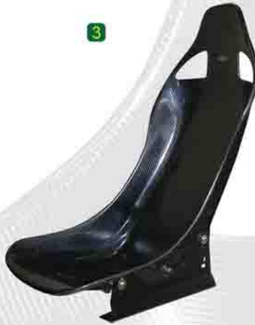
3 Mulsanne B light weight single skin, carbon fibre seat Mass: 3.0kg (approx) R01SI0017
