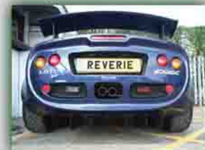
Long five element diffuser
