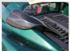
Elise S2 boost tube assembly, provides a high density cold air feed to the engine, reducing intake temperatures R01SB0036
