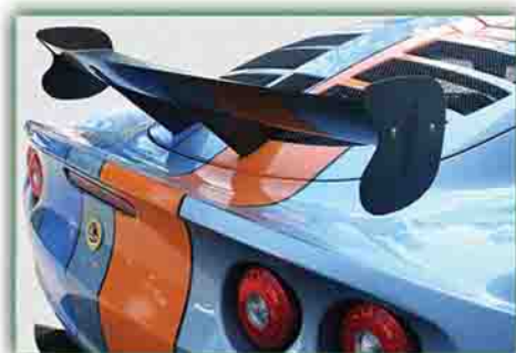
2 Fixed tailgate mounted Curved wing
