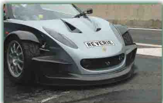
340R carbon fibre / GRP deep spoiler, includes splitter plates and gurney end plates with brake ducts Carbon fibre R01SB0051 GRP R01SB0052 (See images left and page header)
