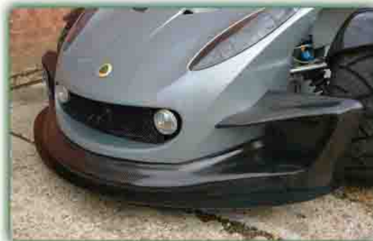
340R carbon fibre / GRP deep spoiler, includes splitter plates and gurney end plates with brake ducts Carbon fibre R01SB0051 GRP R01SB0052 (See images left and page header)
