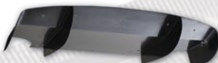
2 Three element, 2.34kg, for standard K Series R01SB0109
