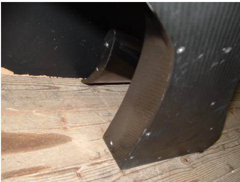
Upper wing ends need dressing back to fit curvature of body neatly.
