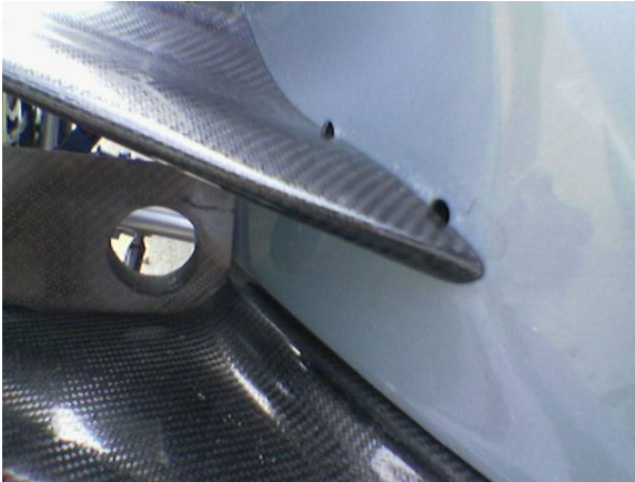
Showing front upper wings need lifting up 5mm
