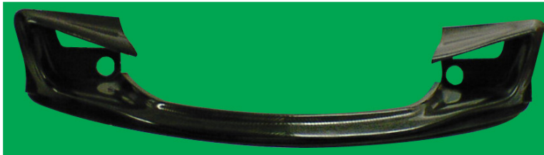
Std height 340r front spoiler shown with optional 58mm brake cooling snorkels fitted
