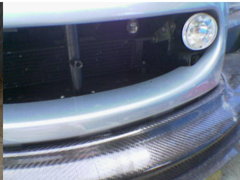
Front spoiler pulled up into position before Bolts tightened fully.
